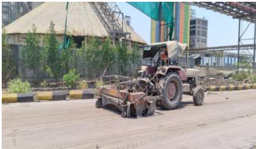
Mechanical Road Sweeper deployed for Road Cleaning
